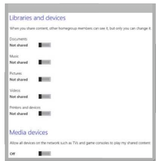
Figure 5-5 To protect files on your device's hard drive from hackers and other intruders, turn off file and printer sharing on your device.
