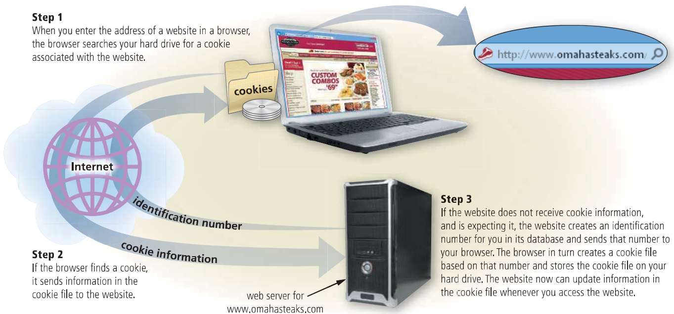
Figure 5-25 This figure shows how cookies work. © Alex Staroseltsev / Shutterstock.com; Source: Omaha Steaks International, Inc.; © iStockphoto / Norman Chan; © Cengage Learning
