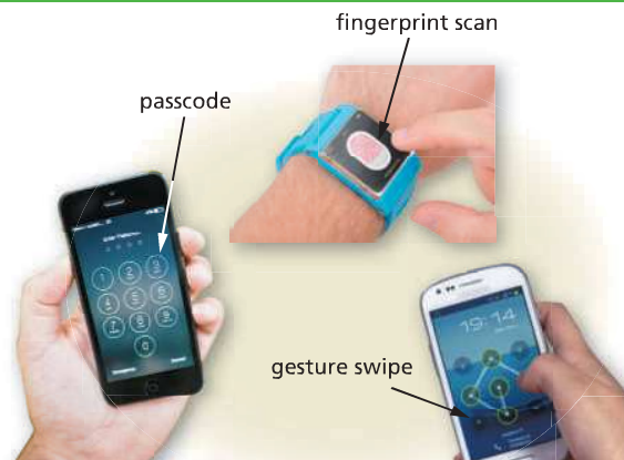
Figure 5-9 Some ways users unlock screens include entering a passcode, scanning a fingerprint, and swiping a gesture.
