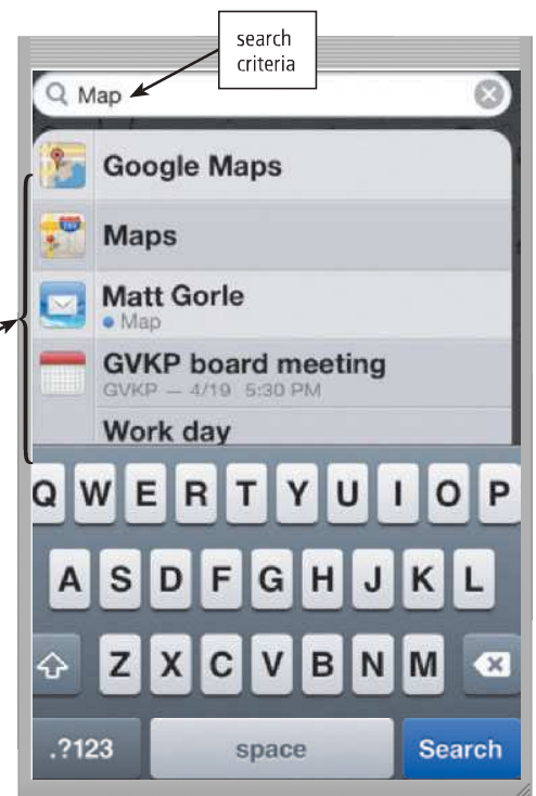
Figure 4-28 This search displays all files on the mobile device that match the search criteria, Map. Notice the search results show map apps, email with a map, and a calendar event.
