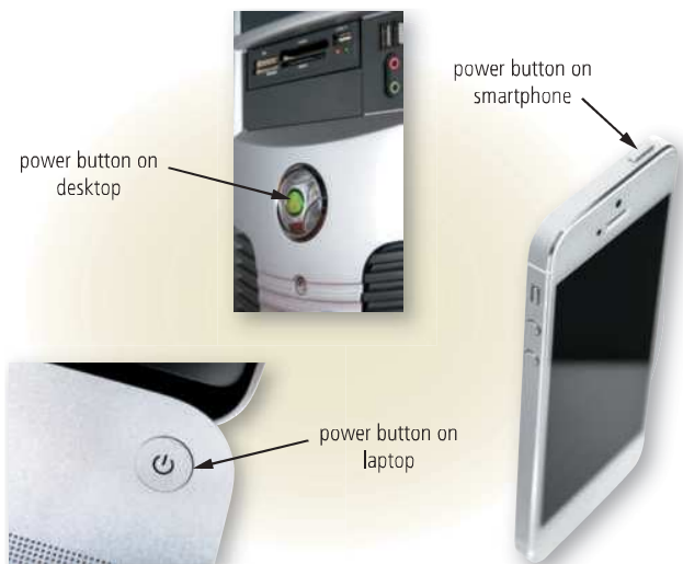
Figure 9-2 Examples of power buttons on computers and mobile devices.
