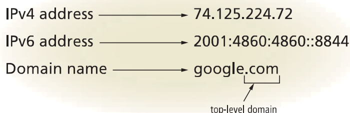
Figure 2-5 The IPv4 and IPv6 addresses, along with the domain name for Google's website.
