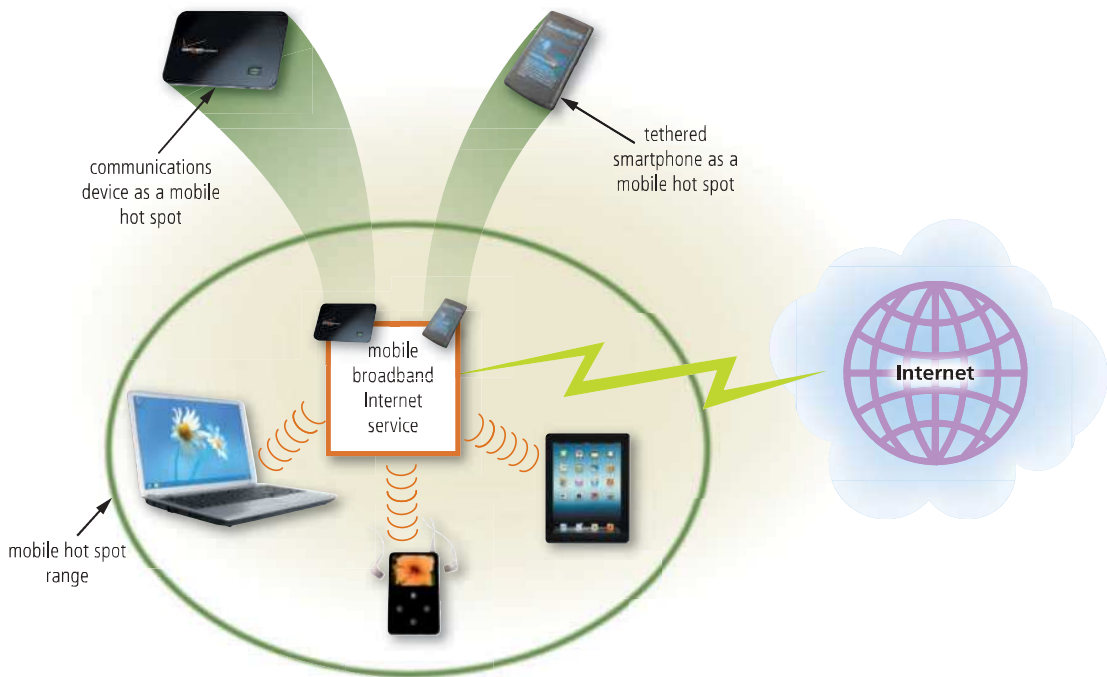
Figure 2-3 You can create a mobile hot spot using a communications device or by tethering a smartphone. Courtesy of Verizon Wireless; © figarro / Can Stock Photo; © iStockphoto / Dane Wirtzfeld; © amfoto / Shutterstock.com; © Alex Staroseltsev / Shutterstock.com; Source: Microsoft; © Cengage Learning
