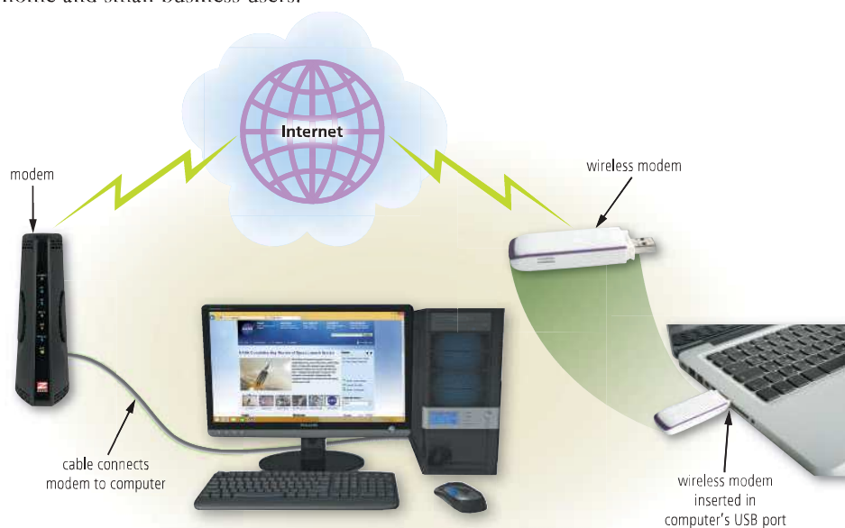
Figure 2-2 Using a modem is one way to connect computers and mobile devices to the Internet.
