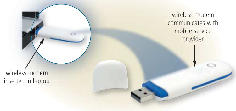
Figure 10-13 Wireless modems allow users to access the Internet wirelessly using a mobile service provider's network. Some manufacturers refer to the type of wireless modem shown in this figure as a USB modem.
