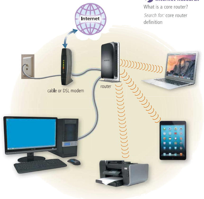
Figure 10-15 Through a router, home and small business networks can share access to a broadband Internet connection, such as through a cable or DSL modem.
