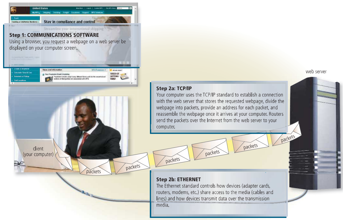
Figure 10-8 This figure illustrates how Internet communications use TCP/IP and Ethernet to ensure that data travels correctly to its destination.
