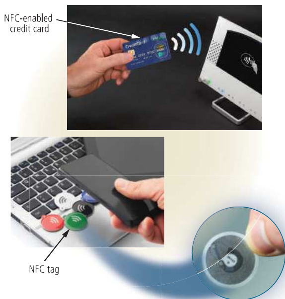
Figure 10-10 Some objects, such as credit cards, are NFC enabled. You also can program NFC tags yourself.
