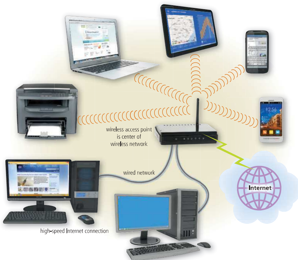
Figure 10-4 Computers and mobile devices on a WLAN may communicate via a wireless access point with a wired LAN to access its hardware, software, Internet connection, and other resources.
