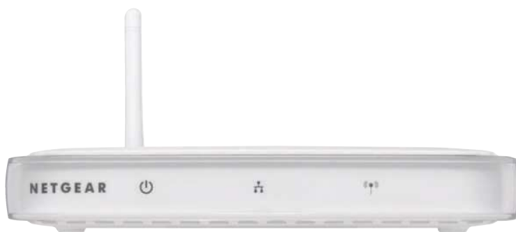
Figure 10-14 Wireless access point.
