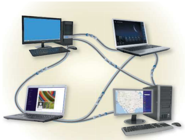
Figure 10-7 As illustrated by the communications in this simplified diagram, each computer or mobile device on a P2P network shares its hardware and software with other computers and mobile devices on the network. Connections can be wired or wireless and may occur through a communications device.
