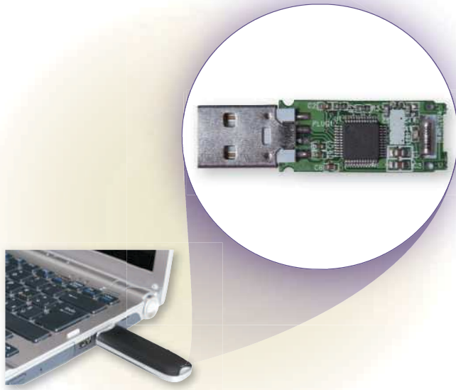
Figure 8-13 A close-up of the flash memory and circuitry inside a USB flash drive.
