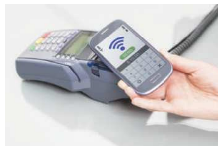
Figure 8-25 This NFC-enabled phone communicates with the NFC reader to send a mobile payment.
