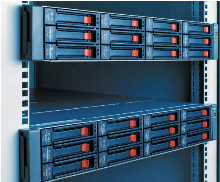
Figure 8-17 Shown here is a rack-mounted RAID chassis, including many integrated hard disks.
