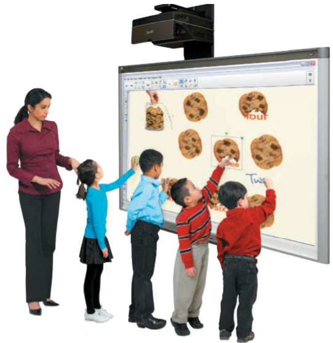
Figure 7-42 Teachers and students can write directly on an interactive whiteboard, or they can write on a slate that communicates wirelessly with the whiteboard.
