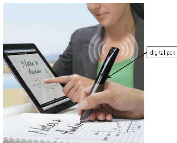
Figure 7-10 Users take notes with a digital pen and then upload the notes to a computer or mobile device, where software translates the notes to typed text.
