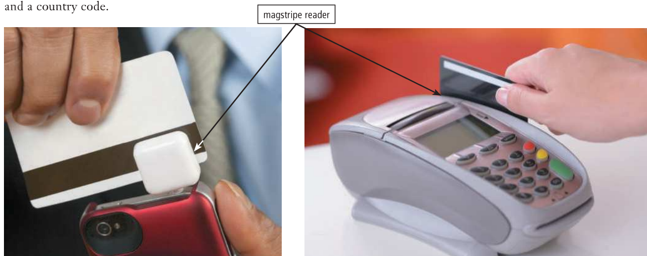
Figure 7-20 A magstripe reader reads information encoded on the stripe on the back of a credit card.
