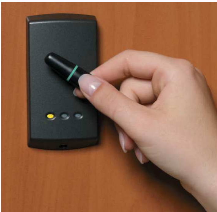
Figure 7-19 This electronic key system locks and unlocks doors using RFID technology.
