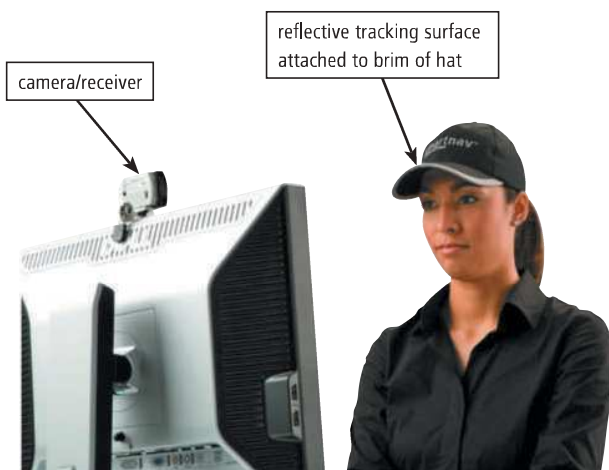
Figure 7-44 A camera/receiver mounted on the monitor tracks the position of the head-mounted pointer, which is the reflective material on the brim of the hat. As the user moves her head, the pointer on the screen also moves.
