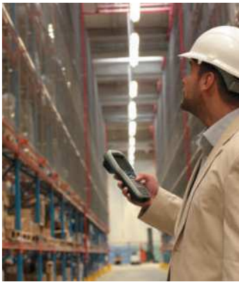
Figure 7-22 An employee in a warehouse uses this data collection device to scan items, which wirelessly transmits information about the scanned item to the store's inventory system.
