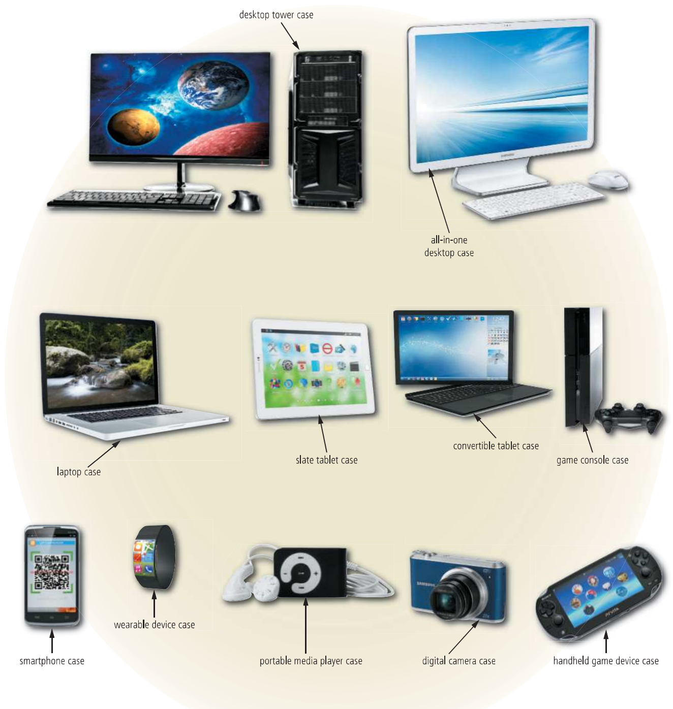
Figure 6-1 Cases for computers and mobile devices are available in a variety of shapes and sizes.
