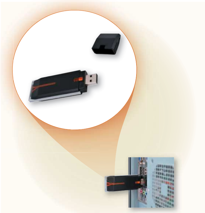
Figure 6-17 A USB adapter inserts into a USB port on a computer or mobile device.
