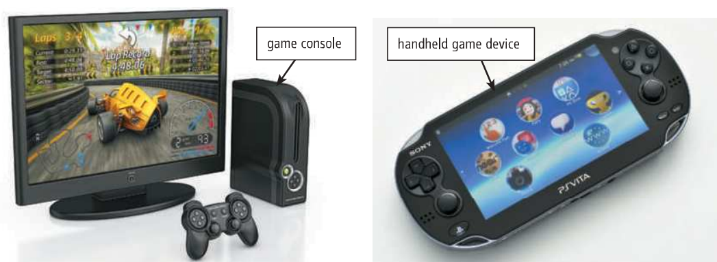
Figure 1-11 Game consoles often connect to a television; handheld game devices contain a built-in screen.
