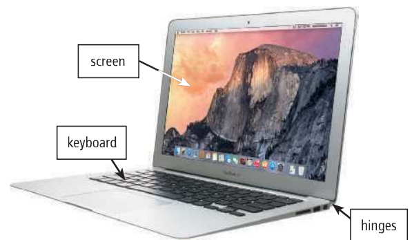
Figure 1-2 A typical laptop has a keyboard in the base and a screen in the lid, with the lid attaching to the base with hinges.
