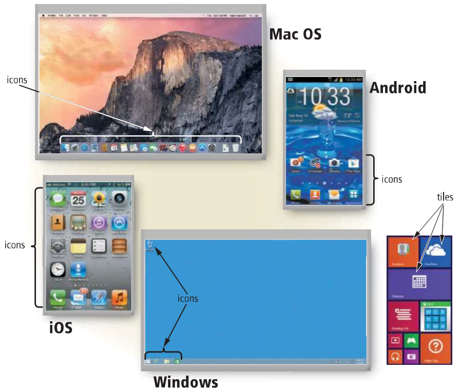
Figure 1-30 Shown here are the Mac OS and Windows operating systems for laptops and desktops and the Android and iOS operating systems for smartphones. You interact with these operating system interfaces by tapping or clicking their icons or tiles. Sources: Apple Inc.; Apple Inc.; Google Inc.; Microsoft.
