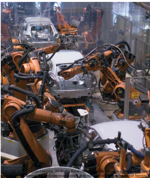
Figure 1-39 Automotive factories use industrial robots to weld car bodies.
