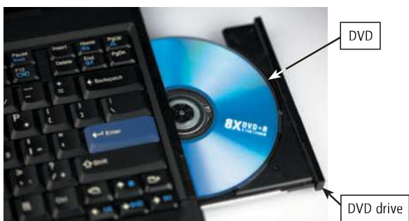
Figure 1-25 You can insert a DVD in a DVD drive on a computer. © iStockphoto / Hanquan Chen
