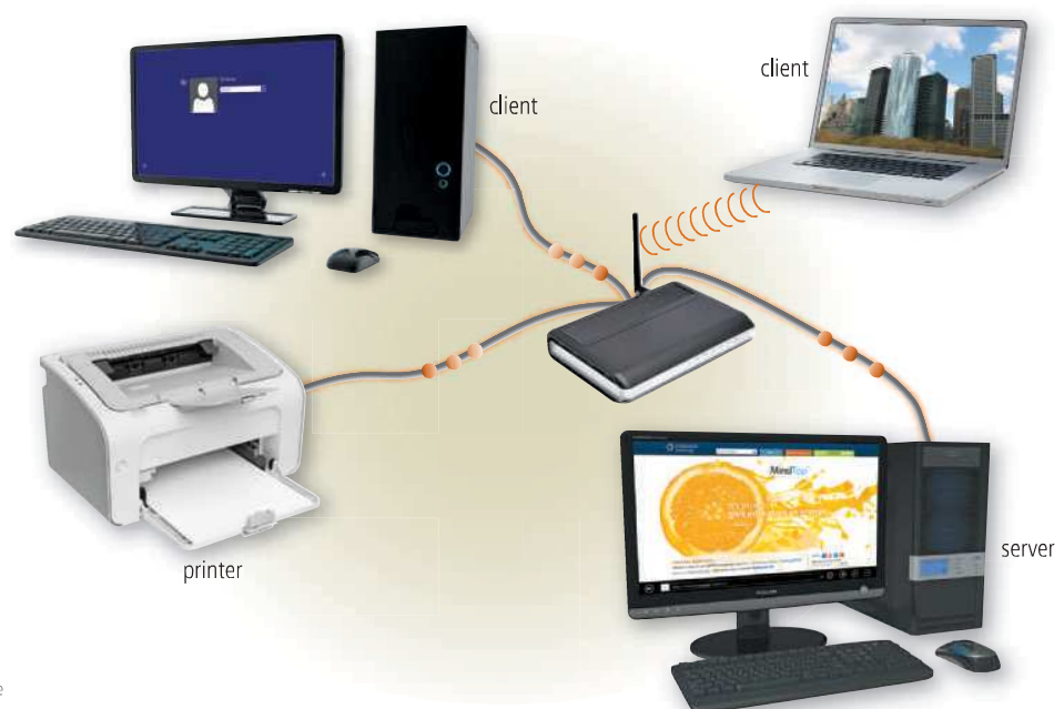
Figure 1-33 A server manages the resources on a network, and clients access the resources on the server. This network enables three separate computers to share the same printer, one wirelessly.
