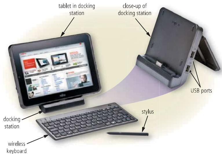
Figure 3-26 Docking stations often are used with tablets and other mobile computers, providing connections to peripheral devices.
