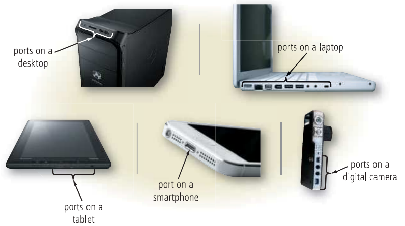
Figure 3-25 Most computers and mobile devices have ports so that you can connect the computer or device to peripherals.
