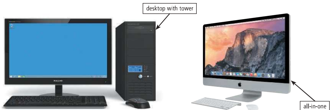
Figure 6 Two different types of desktops. © iStockphoto / Oleksiy Mark; Source: Microsoft; © iStockphoto / hocus-focus; Apple, Inc.
