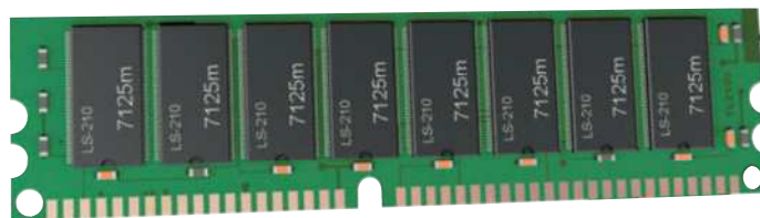
Figure 13 Memory modules contain memory chips.
