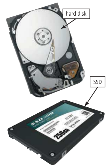
Figure 14 Two different types of storage devices.
